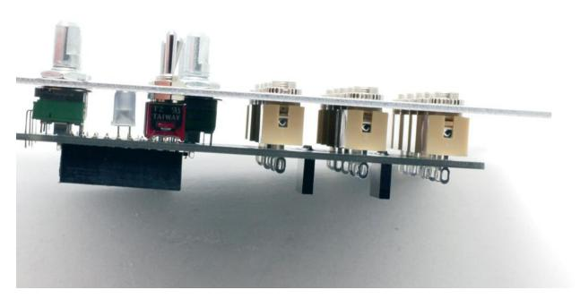
**Make absolutely sure that everything is positioned nicely,** then go ahead and start soldering the control components in place!
