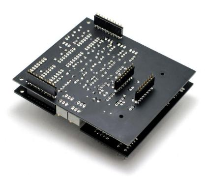
Take the eurorack control board and set it in place over the female header pins sticking up. Begin soldering only a pin or two, checking to make sure it's still lined up straight. When satisfied, solder all of the pins.
