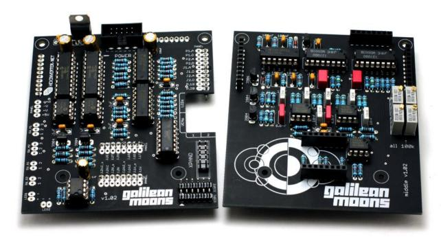
**Now you are done the actual electronics assembly!** I highly recommend going over all of the backs of the PCBs now and making sure there are no shorts or missed soldering points. Once you put the PCB stack together and the panel on, it's pretty daunting to have to take it all apart again to fix a mistake. So, do it right the first time by checking your work over now!
