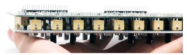
Keeping the panel upside down, you can **solder the legs of each jack** so that they stick up from the PCB when you flip it back.
