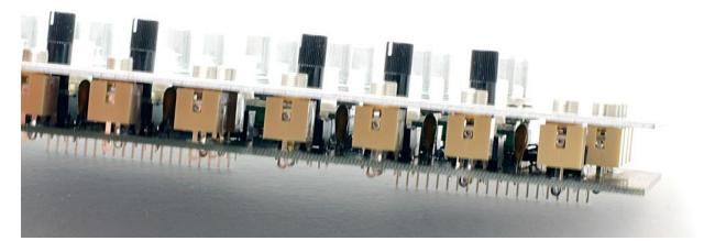
Once you are happy with the way that everything is seated, go ahead and **start soldering all the pins** of the potentiometers and switches. There are a LOT of pins to solder so take your time and don't miss any!
