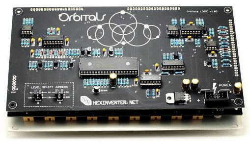
Once everything is tested and you're sure it's working right, **install the knobs as a final step!** Be gentle while installing the knobs and **don't push them all the way down**. Carefully adjust them near the end so they are at the right height and **don't rub on the nut** when turned.
