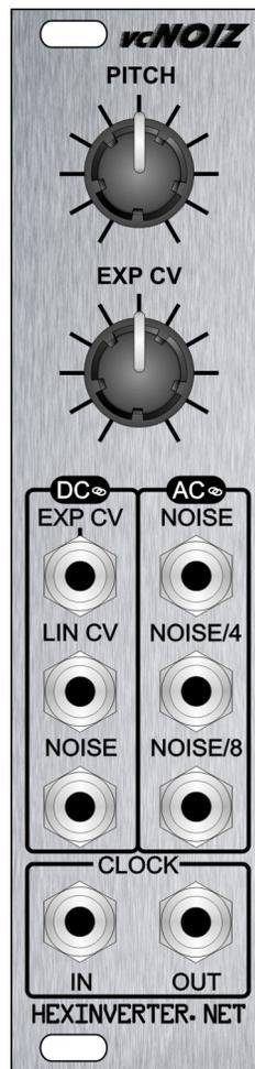
**Pitch Control** -- This controls the base frequency of the noise VCO, just like any other VCO. Express yourself using this control while playing live for some awesome crunchy pitch sweeps! Turning the pitch all the way up will produce white noise at the AC NOISE output. Turning it all the way down will produce sub-audio clicks and pops which are suitable for use as random gates and to trigger events in your system.
